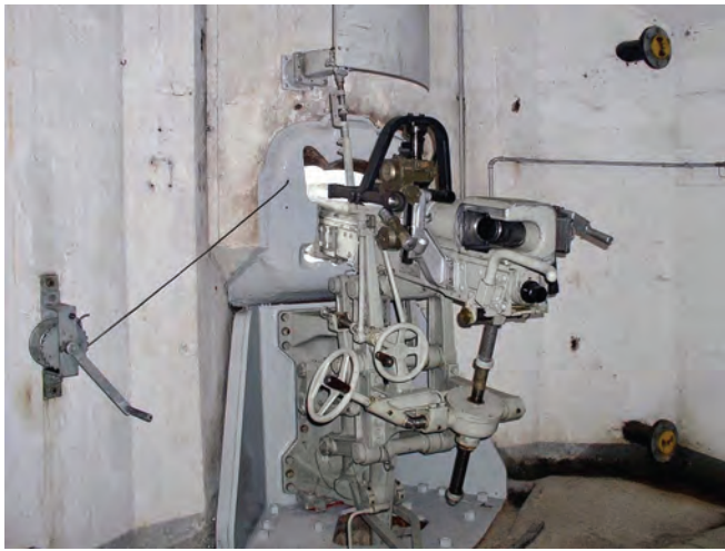
Fort du Scex: A 7.5cm L30 1903/22 gun installed on a lever mount in the 1938/39 "Ermitage Battery".
